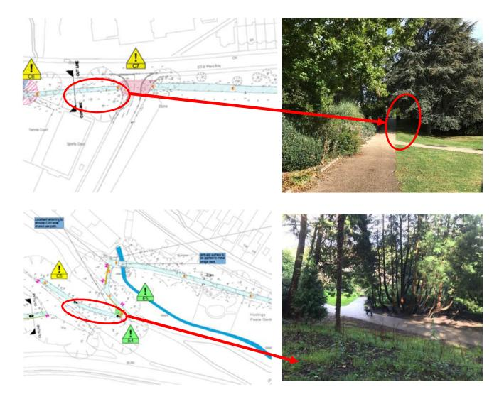
It is recommended that 1.4m high timber post and rail cleft fencing is provided at these locations, consistent with protection of steep banks at other locations along the route.
