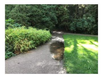
It is recommended that suitable drainage is provided throughout the scheme to ensure that water does not pond within the shared route.
